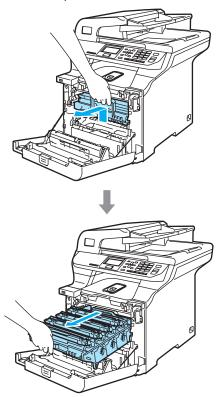
Release the gray lock lever (1) that is on the left side of the machine. Lift the front of the drum unit and pull the drum unit completely out of the machine using the green handles on the drum unit.
